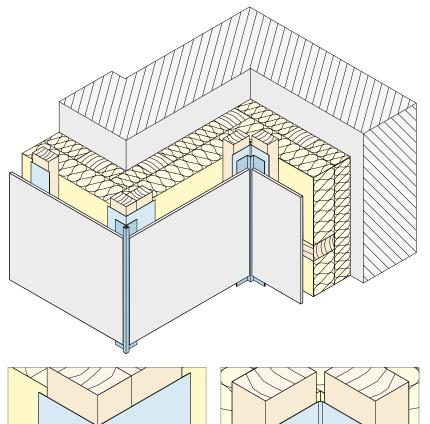
Corner profiles are used for facade design. They cover the cutting edges of the facade boards and form a clean, precise edge.
