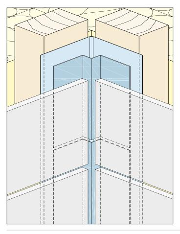
The vertical profile joints of the aluminium corner profiles can also be offset with the joint of the facade cladding. The general use of joint tapes can prevent water from penetrating.
