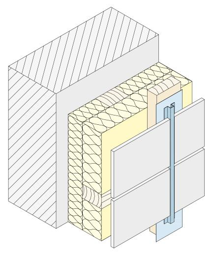
The joint profiles made of aluminium or PVC are used for vertical joints. Ensure that the facade cladding has room for expansion depending on the particular application. The aluminium joint profiles and top hat profiles can be installed on the front or the rearside of the facade cladding.
