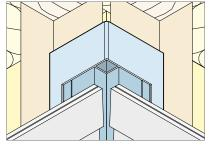
Corner profiles are used for facade design. They fully cover and protect the cutting edges of the facade boards and thus form a clean, precise edge.
