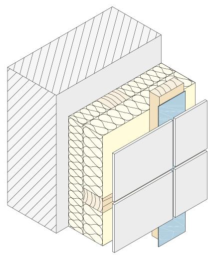
The joint tapes can be used for vertical joints. They decouple the facade cladding and reduce noise transmission. They furthermore reduce water penetration and protect the substructure as well as the insulation from penetrating water. For wooden substructures, the joint tape must overlap at least 5 mm on each side of the substructure.
