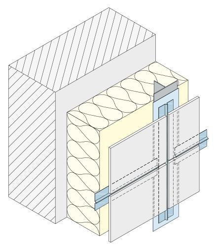
The aluminium joint profile or corrugated profile subtly depicts the joint whilst effectively closing it. The beading along the profile also centres and guides the facade cladding joint. The profiles are therefore available in widths of 6 mm and 9 mm for different joint widths. The corrugated profile may be used horizontally or vertically.
