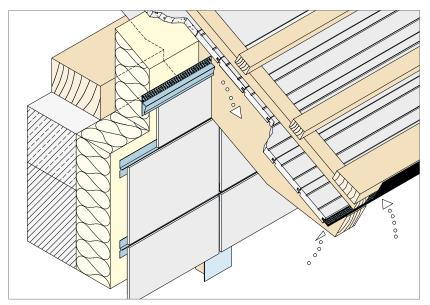
The ventilation profiles 9056 and 9059 are used in the upper facade area and under the window sills. The profiles can be used for board thicknesses of 4 to 6 mm and 8 to 15 mm.
