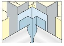
Corner profiles for inside corners form a clean, precise facade cladding stop.
