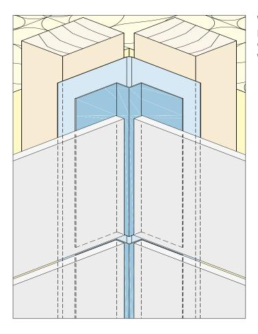
When aluminium corner profiles are used, the vertical profile should may correspond with a joint of the facade cladding. The general use of joint tapes can prevent water from penetrating.
