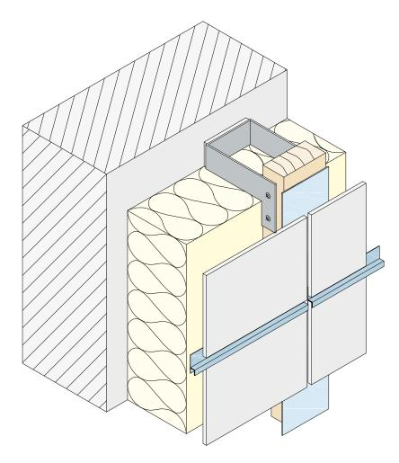
The joint profiles or h-profiles made of aluminium or PVC are used for horizontal joints. They reduce the penetration of moisture. Please ensure that the boards are not placed directly on the profile but that a joint of approx. 5 to 10 mm remains as indicated by the facade cladding manufacturer.
